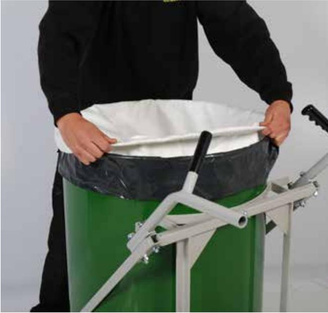
Place the Primary Filter into the top of the drum over the black bag.
