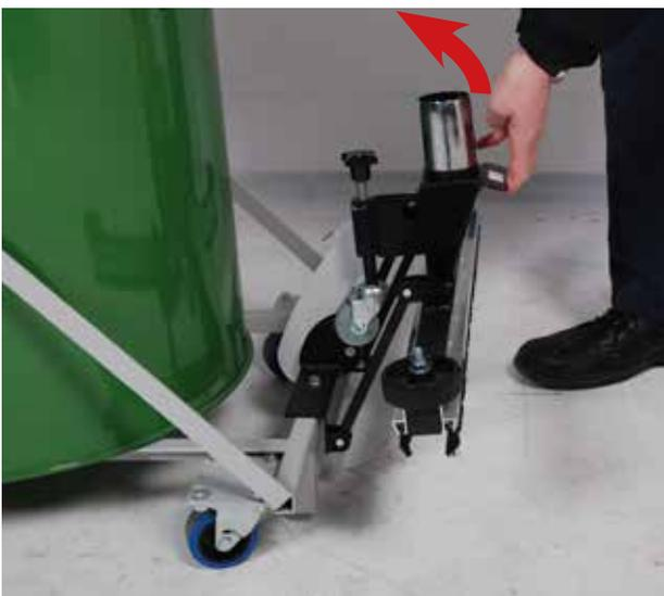
Lift the plate of the Front-Mounted Floor Brush upwards slightly...
