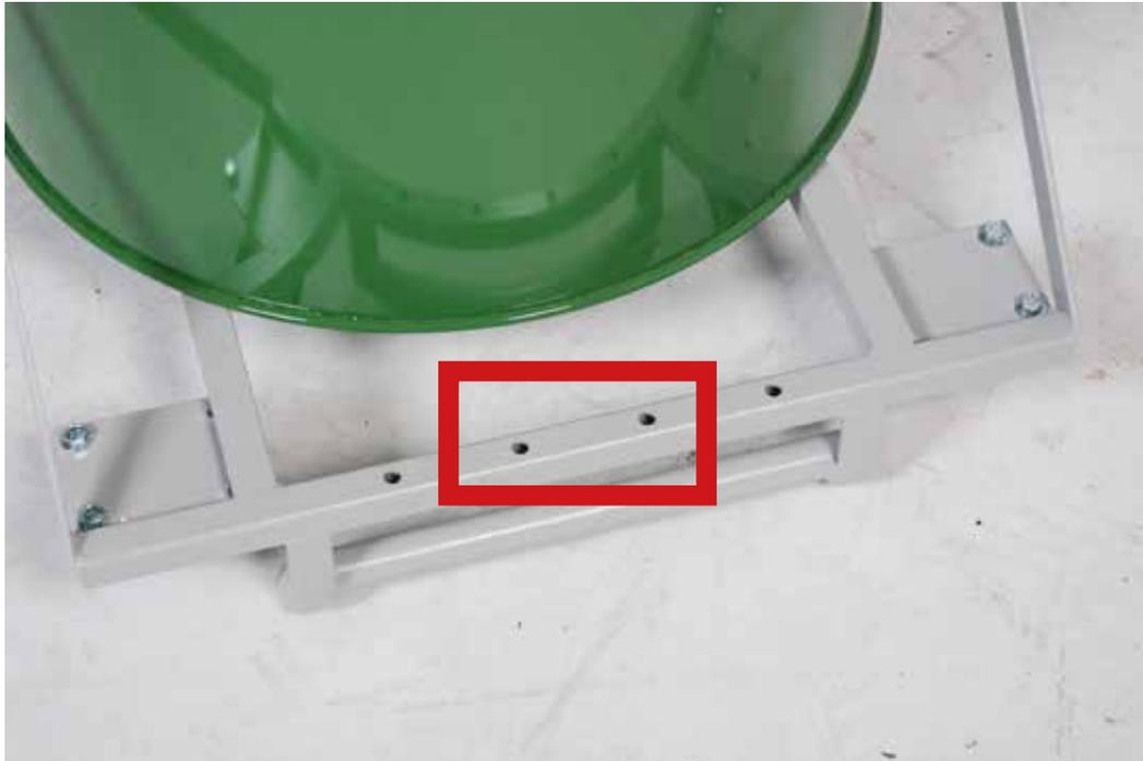
Place a washer onto one of the bolts. Place the bolt through one of the holes in the mounting plate of the Floor Brush and into one of the holes on the front of the cart. Place another washer and a nut on the underside of the bolt. Tighten securely with two open-ended wrenches.
