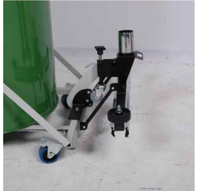
Lift the front plate of the Front-Mounted Floor Brush upwards until the gray retaining catch clicks into place.
