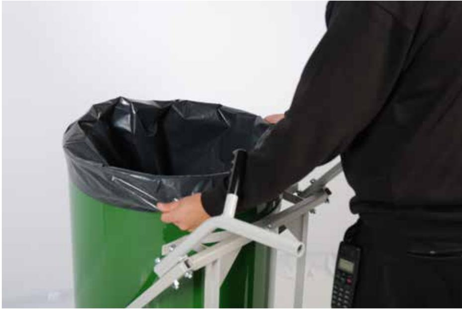
Place a disposable waste bag inside the empty drum and fold the top down over the outside of the drum.
