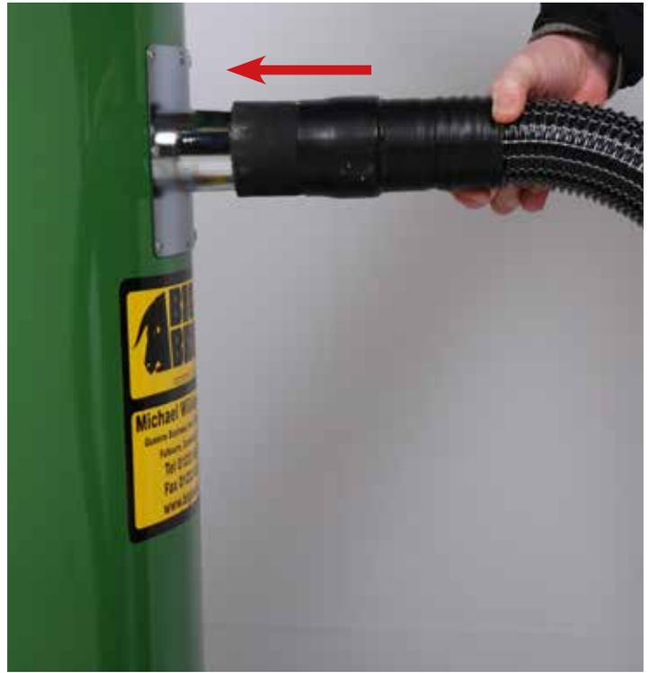
**Attach the link hose to the Front-Mounted Floor Brush and the Drum.**
