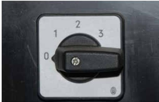
4-position switch for turning on the motors
