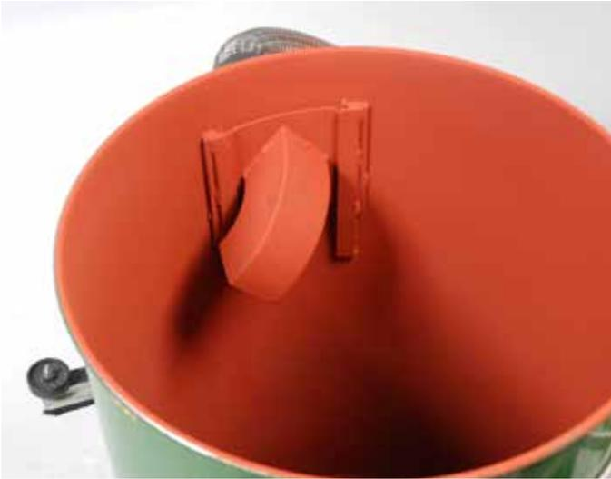
**Optional Lift-Out Spigot correctly positioned - ensure it points downwards into the drum**
