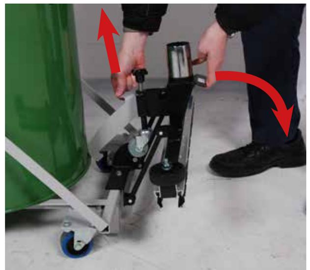
...then lift the gray retaining catch to release the Floor Brush.
